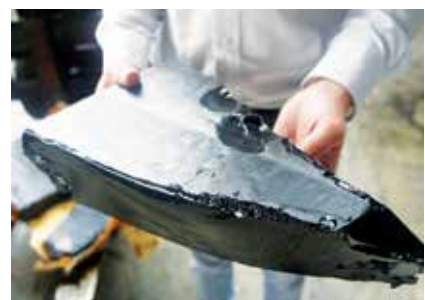
Blown Asphalt produced by the plant
